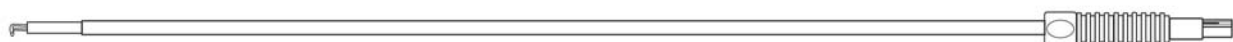
Bipolare Elektroden, Aussen-ø 3 mm, AL 340 mm Bipolar Electrodes, Outside-ø 3 mm, WL 340 mm
